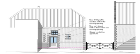
EAST ELEVATION (West Wing) (Garden Wall Removed)
